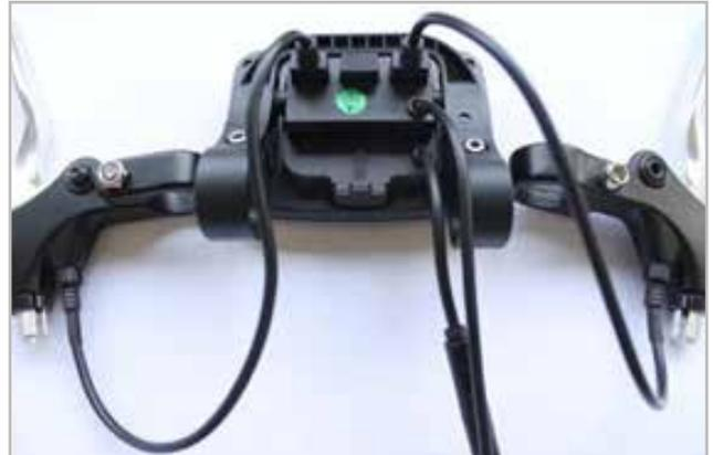
Connect the motor to the LCD display and connect the speed sensor to the motor. The plugs can only go to one place so it's rather kook-proof.
