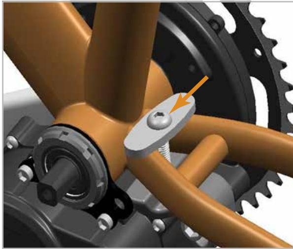
Now go and tighten all bolts to fixing block, securing plate and bottom bracket axle very securely. Use lock-tite liberally here.
