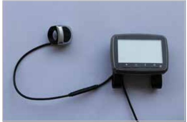
Connect the brake levers if installed to the back of the LCD display. Have a look at the diagram and at the plugs to make sure you don't install them upside down; you'll get an error message on the screen if you do. The left brake connects to the left slot and the right to the right slot. The throttle goes in the middle slot but is not shown here.
